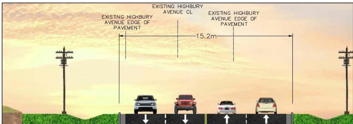
Figure 5.5 Highbury Avenue Widened to the East to 4 Lanes Between Dennis Road & Edgeware Line
