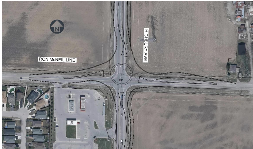
Figure 5.9 Multi-Lane Roundabout Intersection
