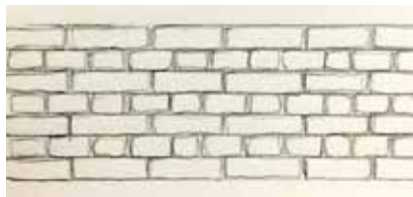
English Bond Alternating rows of stretchers and headers.
