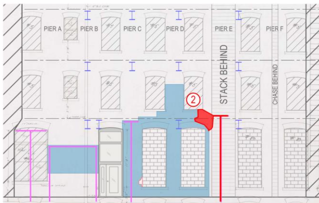
2 MINUTES 44 SECONDS PRIOR TO COLLAPSE BRICK PIECE AT NORTH END OF PIER E DETACHES
